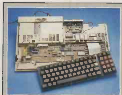
Above: Sinclair ULAs are prominent on the ICL-designed main board. Below: The Xchange ROM cartridge.
