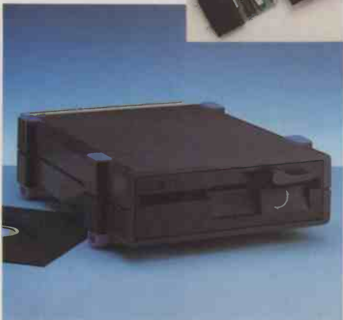
Single disk unit fitted with 5 1/4 inch drives and (inset) the Q-Disk controller.
