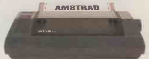
Optional 80 column dot matrix printer DMP-1. Operates at up to 50 characters per second.
