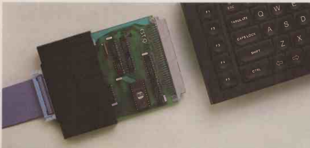
An IEEE-488 interface slips discreetly into place.
